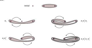
We use the braid generator notation:  $\sigma_i$  means the clockwise interchange of the *i*th and (i + 1)th rod. (Inverses are counterclockwise.)
